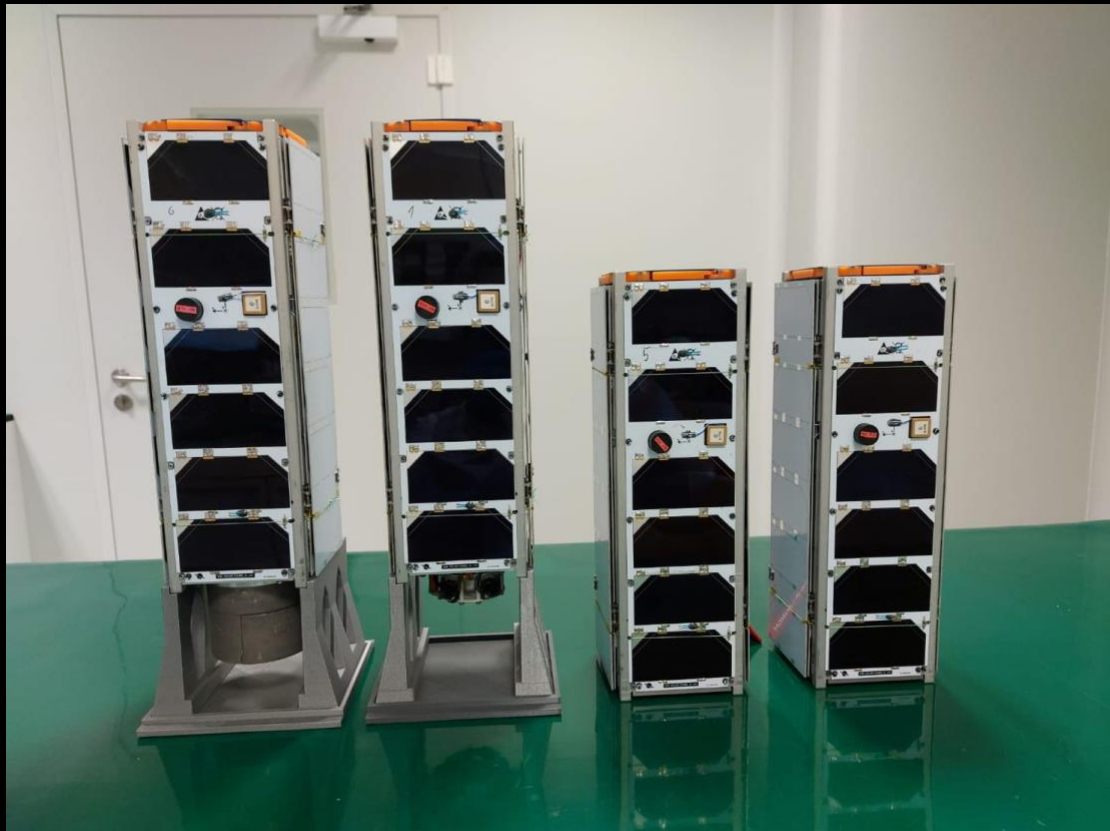
Figure 1. SatRevolution developed four 3U CubeSats that weigh around 4 kg in 2021. They will be sequentially deployed to the 550 km Sun Synchronous orbit (SSO). The CubeSat that carries Tensor Tech's spherical-motor-based ADCS is the second one counting from the left. This ADCS is mounted right in the bottom part of the CubeSat. (tuna-can)
